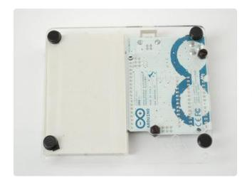
Finally, place four bumpers on the bottom!
