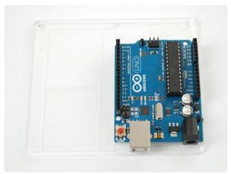
Place the Arduino on top, it should slide onto the bolts
