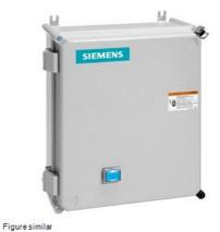
Reversing motor starter, Size 2 1/2, Three phase full voltage, Amb. compensate bimetal OLR, Contactor amp rating 60A, 110V 50Hz / 120V 60Hz coil, Non-combination type, Enclosure type 4X fiberglass, Water/dust tight noncorrosive
