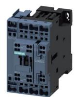
Contactor, AC-1, 40 A/400 V/40  $^\circ\text{C},$  S0, 4-pole, 110 V DC, 1 NO+1 NC, Spring-type terminal
