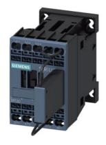
traction contactor, AC-3 12 A, 5.5 kW / 400 V 110 V DC, 0.7-1.25\*US with integrated suppressor diode 3-pole, size S00 spring-type terminal suitable for PLC outputs not expandable with auxiliary switch
