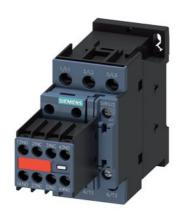
Power contactor, AC-3 12 A, 5.5 kW / 400 V 2 NO + 2 NC, 110 V AC, 50 Hz 120 V, 60 Hz, with plugged-in varistor, 3-pole, Size S0 Screw terminal Captive auxiliary switch
