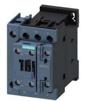
Contactor, AC-3, 11 kW/400 V 110 V AC/50/60 Hz 4-pole, 2 NO+2 NC, Size S0 Screw terminal 1 NO+1 NC integrated
