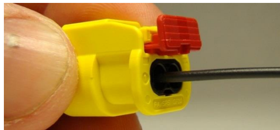
Cable seal terminal orientation feature (proper orientation)
