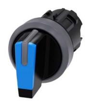
Selector switch, illuminable, 22 mm, round, plastic with metal front ring, blue, selector switch, short, 3 switch positions I>O<II, momentary contact on the left, latching on the right, actuating angle 2x45°, 10:30h/12h/13:30h
