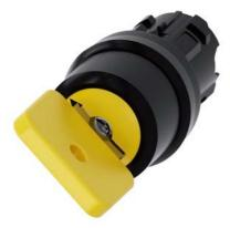
Key-operated switch O.M.R, 22 mm, round, plastic, lock number 73033, yellow, with 2 keys, 2 switch positions O-I, latching, actuating angle 90°, 10:30h/13:30h, Key removal O+I
