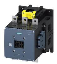
Contactor, AC-1, 690 A/690 V/40  $^\circ\text{C},$  S12, 3-pole, 200-277 V AC/DC, F-PLC-IN with varistor, 2 NO+2 NC, Connection rail/ screw terminal
