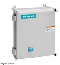
Non-reversing motor starter, Size 3 1/2, Three phase full voltage, Amb. compensate bimetal OLR, Contactor amp rating 115A, Non-combination type, Enclosure type 4X fiberglass, Water/dust tight noncorrosive
