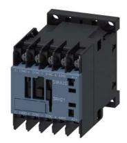
Coupling contactor relay railway 2 NO + 2 NC, 24 V DC, 0.7  $\dots$  1.25\* US, with varistor integrated, Size S00, ring cable lug connection
