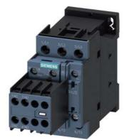
Power contactor, AC-3 32 A, 15 kW / 400 V 2 NO + 2 NC, 230 V AC 50/60 Hz, 3-pole Size S0, screw terminals Removable auxiliary switch
