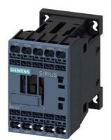
Contactor relay, 4 NO, 48 V DC, Size S00, Spring-type terminal
