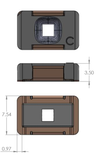
Mechanical design features without solder clip
