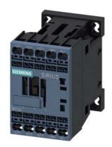
power contactor, AC-3 12 A, 5.5 kW / 400 V 1 NO, 110 V DC 0.7-1.25\* US, with varistor integrated, 3-pole Size S00, Spring-type terminal
