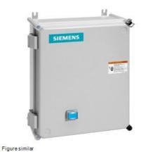
Non-reversing motor starter, Size 2 1/2, Three phase full voltage, Amb. compensate bimetal OLR, Contactor amp rating 60A, Non-combination type, Enclosure type 4X fiberglass, Water/dust tight noncorrosive
