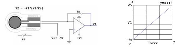
2. Using a fixed resistor R1 in a voltage divider configuration for an output V2 that increases with respect to added force. Use this circuit topology for budget or power-conscious applications.
