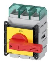
SENTRON, Molded case switch 3LD5 UL, Emergency switching-off, 3-pole, certified according to UL489 UL60947-4-1 and IEC60947-3, UL: 100A, SCCR 65kA at 480VAC, Operating power at 480VAC 3-phase: 60hp, IEC: 100A, Operating power at AC-23A at 400V: 45kW, front-mounted, rotary operating mechanism, red/yellow, 4-hole mounting of the handle, incl. terminal covers for the infeed side
