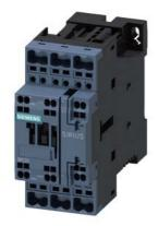
power contactor, AC-3 9 A, 4 kW / 400 V 1 NO + 1 NC, 220 V DC 3-pole, Size S0 Spring-type terminal
