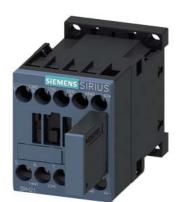
Coupling contactor relay, 3 NO + 1 NC, 24 V DC, 0.85  $\dots$  1.85\* US, with varistor plugged on, Size S00, screw terminal
