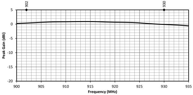
Figure 4. ANT-915-VHETH Antenna Peak Gain
