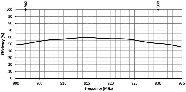
Figure 6. ANT-915-VHETH Antenna Radiation Efficiency
