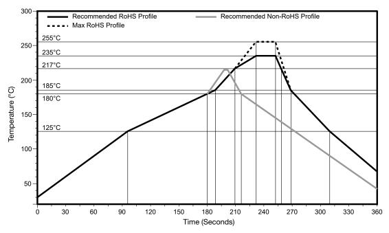
Figure 11. Solder Profile for the ANT-915-VHETH Antenna
