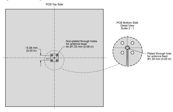
Figure 10. ANT-915-VHETH Antenna Placement on PCB
