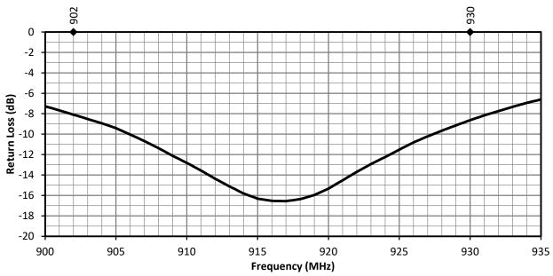
Figure 3. ANT-915-VHETH Antenna Return Loss
