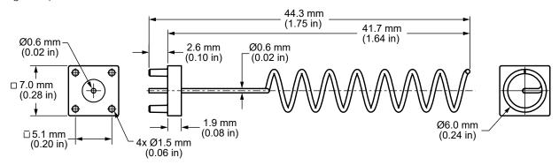
Figure 1. ANT-915-VHETH Antenna Dimensions
