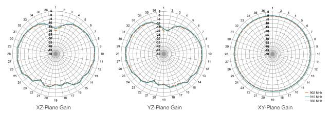
Figure 7. ANT-915-VHETH Antenna Radiation Patterns
