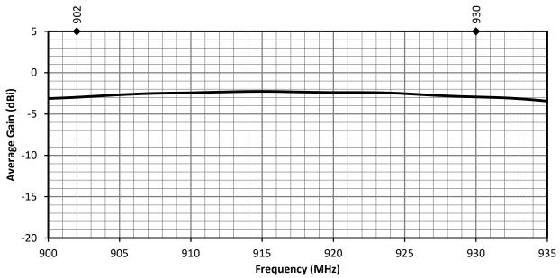
Figure 5. ANT-915-VHETH Antenna Average Gain
