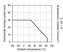
Luminous Intensity vs. Ambient Temperature
