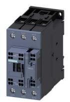
power contactor, AC-3 40 A, 18.5 kW / 400 V 1 NO + 1 NC, 400 V AC 50 Hz, 3-pole, Size S2, Spring-type terminal
