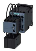
Capacitor contactor, AC-6b 12.5 kVAr, / 400 V 2 NC, 110 V AC, 50/60 Hz 3-pole, Size S00 screw terminal
