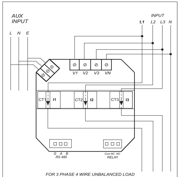
It is recommended that the wires used for connections to the instrument should have lugs soldered at the end. That is, the connections should be made with Lugged wires for secure connections. The Maximum diameter of the lug should be 7.0 mm and maximum thickness 3.5 mm.
