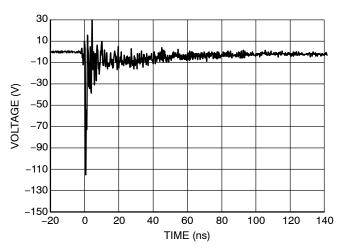
Figure 2. Typical IEC61000-4-2 -8kV Contact ESD Clamping Voltage
