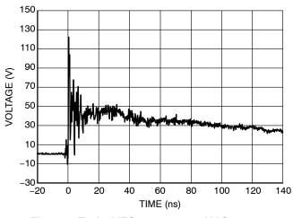
Figure 1. Typical IEC61000-4-2 +8kV Contact ESD Clamping Voltage
