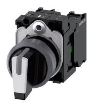
Selector switch, illuminable, 22 mm, round, plastic with metal front ring, white, selector switch, short, 3 switch positions I-O-II, latching, actuating angle 2x45°, 10:30h/12h/13:30h, with holder, 1 NO, 1 NO, screw terminal, with laser labeling, upper case and lower case, always upper case at the beginning of the word
