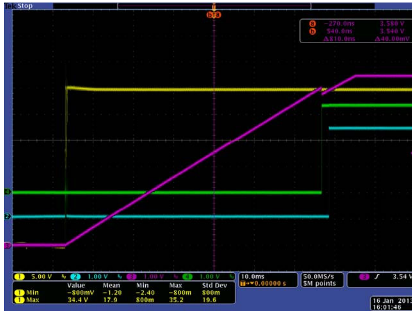
Figure 6. NCN5150 Startup Sequence
