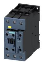
contactor, AC-3, 65 A/400 V/60  $^\circ C$  S2, 3-pole, 83-150 V AC/DC, F-PLC-IN, with varistor, 1 NC, screw terminal
