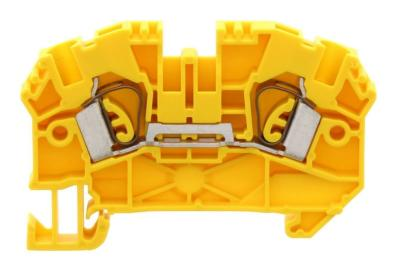
Feed-through terminal, Tension-spring connection, Mounting type: Mounting rail TS 35/7.5, Rated cross-section: 4 mm², Width: 6.1 mm, Colour: Yellow
