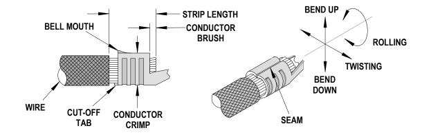
The above terminal drawing is a generic terminal representation. It is not an image of any terminal listed in the scope.
