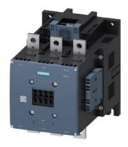
power contactor, AC-3 400 A, 200 kW / 400 V AC (50-60 Hz) / DC operation 200-277 V AC/DC auxiliary contacts 2 NO + 2 NC 3-pole, frame size S12 busbar connections drive: electronic with PLC interface 24 V DC spring-loaded terminal
