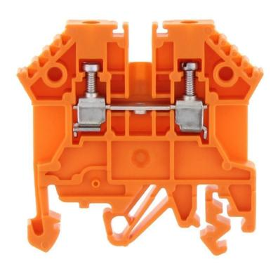
Feed-through terminal, Screw connection, Mounting type:Mounting rail TS 35/7.5 and TS 32, Rated cross-section: 2.5 mm², Width: 5 mm, Colour: Orange
