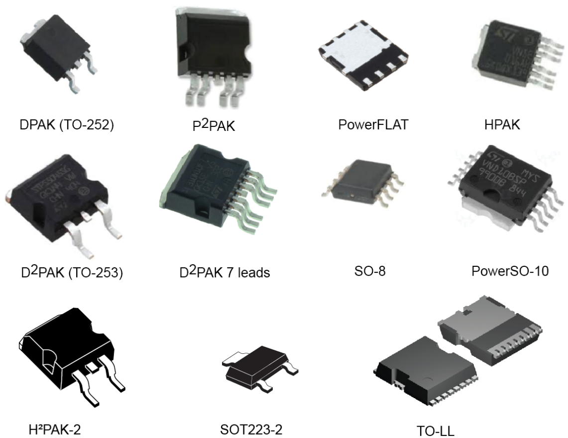
Figure 1. Examples of SMD packages
