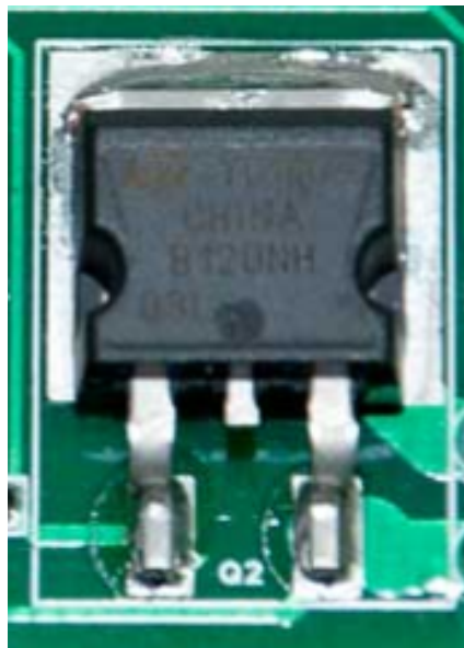
Figure 9. Example of a correctly soldered D 2 PAK package on PCB
