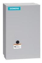
Mechanically held lighting contactor, Contactor amp rating 100A, 0 N.C. / 3 N.O. poles, 220VAC 50HZ/240VAC 60HZ coil, Non-combination type, Enclosure NEMA type 1, Indoor general purpose use
