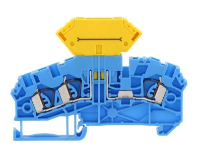
Disconnect terminal, Tension-spring connection, Mounting type: Mounting rail TS 35/7.5, Rated cross-section: 2.5 mm², Width: 5.1 mm, Colour: Blue
