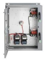
Pump control panel, Duplex controller NEMA size 1 Solid-state overload relay, OLR amp range 0.75-3.4A, 120 VAC coil, Fusible disconnect HOA Sel Sw. and Start P.B., Enclosure NEMA type 3/3R,12 Weather proof outdoor use
