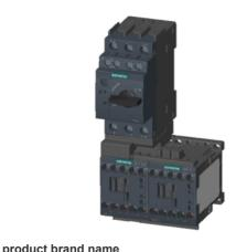
Fuseless motor starter Reversing operation 600VAC Size S00 0.35-0.5A 24V DC screw connection For screw mounting Or 35 mm rail-mounting Type of coordination 2 IQ = 150 KA Also full fills type Of coordination 1 1NO+1NC (MSP) 1NC (per contactor)
