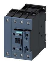
Contactor, AC-1, 60 A/400 V/40 °C, S2, 4-pole, 220 V AC, 50/60 Hz, 1 NO+1 NC, screw terminal
