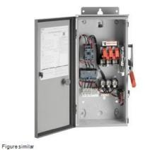
Slim Line Pump Control Panel NEMA size 1 Three phase full voltage Solidstate overload relay OLR amp range 5.5-22A 110/120V 50/60Hz Coil 30A fusible disconnect 30A/600V fuse clip 1NC / 1NO auxiliary contacts HOA Sel. Sw. <(>&<)> Start/Stop 3-point power terminal block 3-point control terminal block 3-point ground lug Enclosure NEMA type 3/3R Weather proof outdoor use
