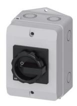
SENTRON, Switch disconnector 3LD, main switch, 3-pole, lu: 25 A, Operating power / at AC-23 A at 400 V: 9.5 kW, molded-plastic encapsulation for inch cable gland, 1 NC, 1 NO, rotary operating mechanism, black
