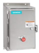
Non-reversing motor starter, Size 0, Single phase full voltage, Solid-state overload relay, OLR amp range 5.5-22A, Non-combination type, Encl. type 4X 304 S. Steel, Water/dust tight noncorrosive, Standard width enclosure
