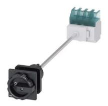
SENTRON, Switch disconnector 3LD, main switch, 4-pole, lu: 25 A, Operating power / at AC-23 A at 400 V: 9.5 kW, floor mounting with door coupling, rotary operating mechanism, black, central mounting 22.5 mm of the handle
