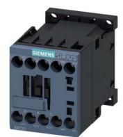
power contactor, AC-3 9 A, 4 kW / 400 V 1 NO, 24 V DC, 0.7-1.25\*US with integrated suppressor diode 3-pole, size S00, screw terminal suitable for PLC outputs not expandable with auxiliary switch
