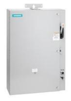
Pump control panel, Size 3, Three phase full voltage, Solid-state overload relay, OLR amp range 25-100A, 110-120/220-240VAC 60Hz coil, Standard type contactor, 200A fusible disconnect, 200A/600V fuse clip, HOA Sel Sw. <(>&<)> Start P.B., Enclosure NEMA type 3/3R, Weather proof outdoor use
