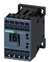
Coupling contactor relay, 3 NO + 1 NC, 24 V DC, 0.7  $\dots$  1.25\* US, with integrated suppressor diode, Size S00, Spring-type terminal suitable for PLC outputs
