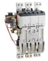
Mechanically held lighting contactor, Contactor amp rating 400A, 0 N.C. / 2 N.O. poles, 220VAC 50HZ/240VAC 60HZ coil, Non-combination type, Enclosure NEMA type (open), No enclosure
