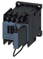
traction contactor, AC-3 12 A, 5.5 kW / 400 V 24 V DC 0.7-1.25\* US, with suppressor diode integrated 3-pole, size S00 ring cable lug connection suitable for PLC outputs not expandable with auxiliary switch
