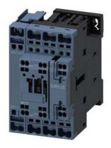
Contactor, AC-1, 35 A/400 V/40 °C, S0, 4-pole, 24 V AC, 50/60 Hz, 1 NO+1 NC, Spring-type terminal
